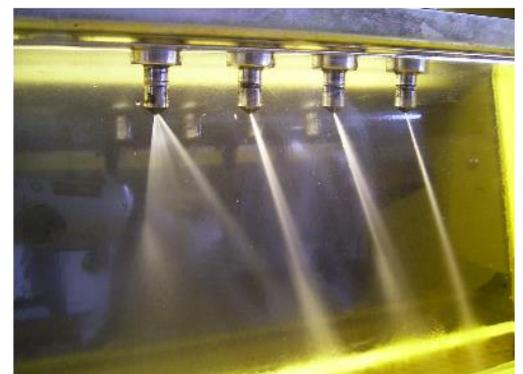
**Fact:** If you had 6 injectors and 6 different deliveries, with the help of the EMS the engine would run correctly. With 6 different spray patterns and 6 correct deliveries, the engine would run badly.
